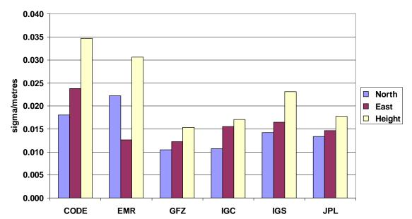
**Figure 4:** Static GIPSY PPP RMS (stations AUCK, BRUS, USUD, WILL) with IGS, AC orbit/clock solutions and the new clock combination *IGC* for GPS Wk 0995 (corrected for daily geocenter origin offsets; IGC represents the new clock combination, adopted by IGS on November 5, 2000)
