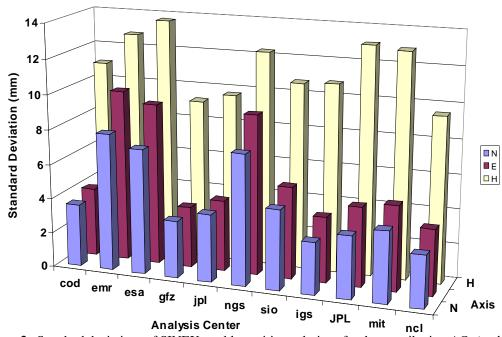
**Figure 3**. Standard deviations of SINEX weekly position solutions for the contributing *ACs* (*cod, emr, esa, gfz, jpl, ngs, sio*), the IGS weekly combined products (*igs*) and the GNAAC combinations (*JPL, mit, ncl*) with respect to the IGS cumulative SINEX product during 1996-2000 (GPS Week 0837-1081).
