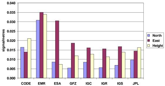
**Figure 5:** Static BERNESE PPP RMS (stations BRUS, WILL, TOW2), with IGS, IGR, AC orbit/clock solutions and the new clock combination IGC for GPS Week 1081 (September 24-30, 2000; corrected for a weekly geocenter origin offset)
