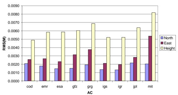
**Figure 9:** Static GPS Pace PPP repeatability at 36 Reference frame stations (RS) with respect to weekly average positions, using IGS, IGR and AC orbit/clock solutions for GPS Week 1516 (January 25 - 31, 2009)
