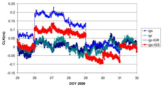
**Figure 12.** 24-h linear regression clock residuals for GPS Pace PPP station clock solutions with IGS Final (*igs*) and IGS Rapid (*igr*) orbits/clocks at the European RS BRUS during the GPS Week 1516. Also shown are the PPP clock solution differences with respect to the IGS Final (*IGS*) and Rapid (*IGR*) combined station clocks with no offsets or drifts removed.
