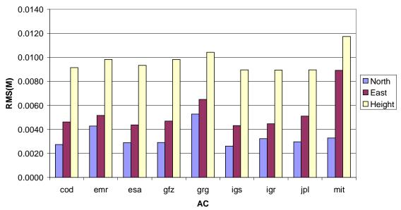
**Figure 8:** Static GPS Pace PPP RMS at 36 Reference frame stations (RS) with IGS, IGR and AC orbit/clock solutions for GPS Week 1516 (January 25-31, 2009; *corrected* for daily geocenter origin/scale offsets)
