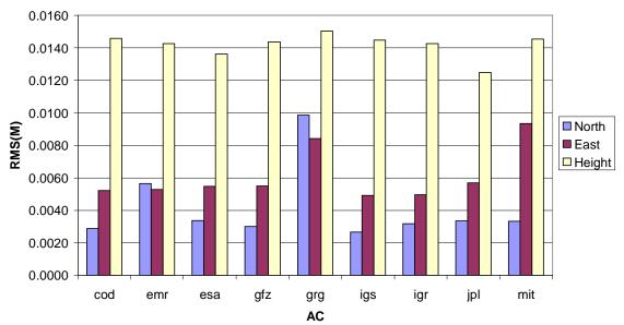
**Figure 7:** Static GPS Pace PPP RMS at 36 Reference frame stations (RS) with IGS, IGR and AC orbit/clock solutions for GPS Week 1516 (January 25 - 31, 2009; no geocenter origin/scale offset corrections)
