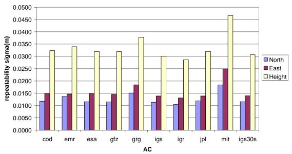
**Figure 10:** Average kinematic (navigation) GPS Pace PPP repeatability at 36 Reference frame stations (RS) with respect to weekly average positions, using IGS, IGR and AC orbit/clock solutions for GPS Week 1516 (January 25 - 31, 2009)
