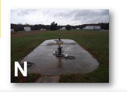
Antenna ARP ~ 50 cm above concrete pad (zero tilt) ○ 10 cm Sokkia
