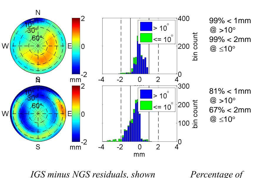
with respect to azimuth and elevation angle (lefthand circular plots) and as a histogram (righthand). Vertical bars in histogram denote 1mm and 2mm bounds for IGS AWG approval.
