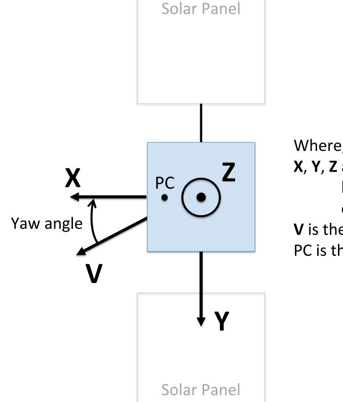
X, Y, Z are unit vectors defining spacecraft body fixed coordinate system, with origin at the center of gravity, **V** is the velocity vector,
