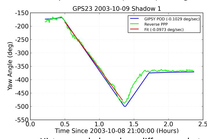
Yaw angle is between the velocity vector V and +X
