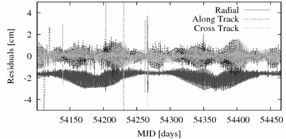
**Fig. 2** Orbit differences for models ALB-8 – ALB-0 for satellite SVN36 for the year 2007.
