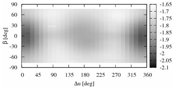
**Fig. 3** Radial residuals (in cm) between the models ALB-8 and ALB-0 for SVN36 in a Sun-fixed reference frame.
