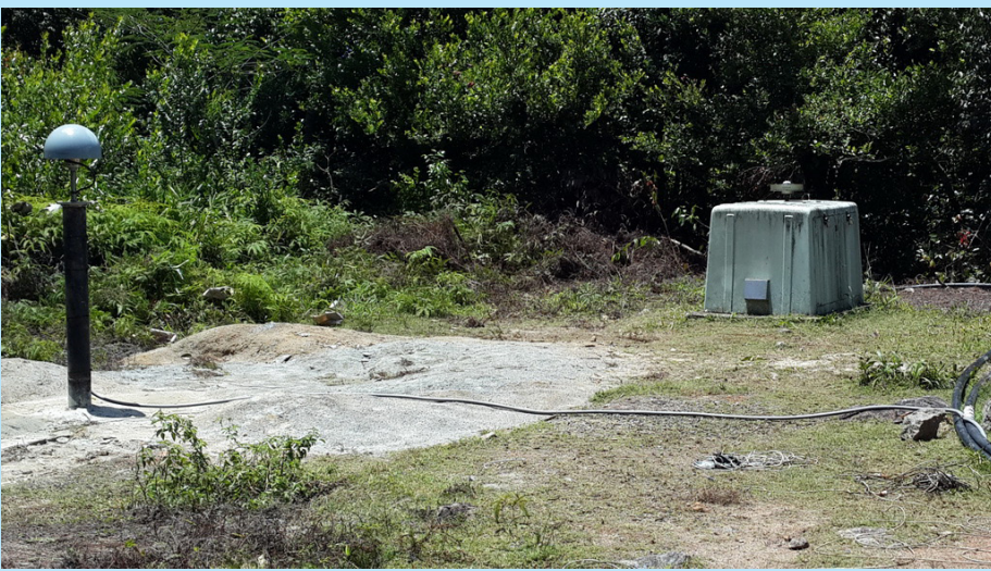
The new SEY2 monument is located 25 feet from the original SEY1 antenna. The SEY1 monument will be demolished when UCSD visits the station to conduct maintenance on their borehole seismometers in early 2016.
