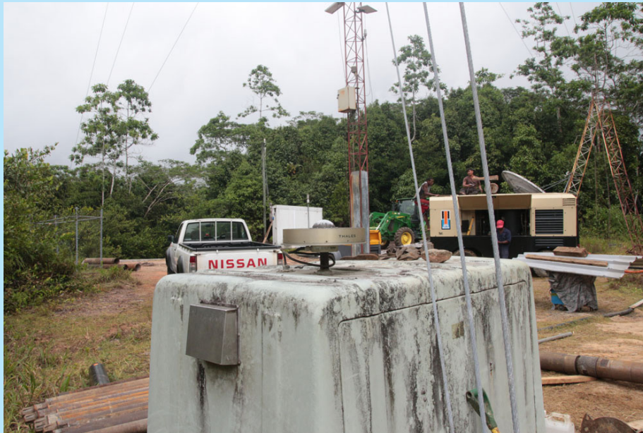
Photos shows original SEY1 antenna with guy wires that supported a nearby cellular communications tower. The tower was no longer in use and was demolished after the SEY2 monument was built. Awkward seismic well-head access (difficult to reoccupy location precisely, and IDA coordination required) were a compelling case for a new monument.
