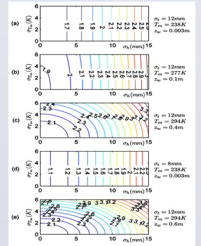
Fig. 5: The achievable accuracies of PWV in different climatic conditions defined by  $\sigma_T$  (RMS of PPP-ZTD),  $T_m$  and  $\sigma_w$  (ZWD): (a & d) represent polar regions; (c & e) represent tropical or subtropical regions; and (b) represents the moderate conditions. Fig. 5d differs from Fig. 5a assuming PPP-ZTD is more accurate (smaller  $\sigma_T$ ), while Fig. 5e differs from Fig. 5c assuming higher relative humidity (larger  $\sigma_w$ ).
