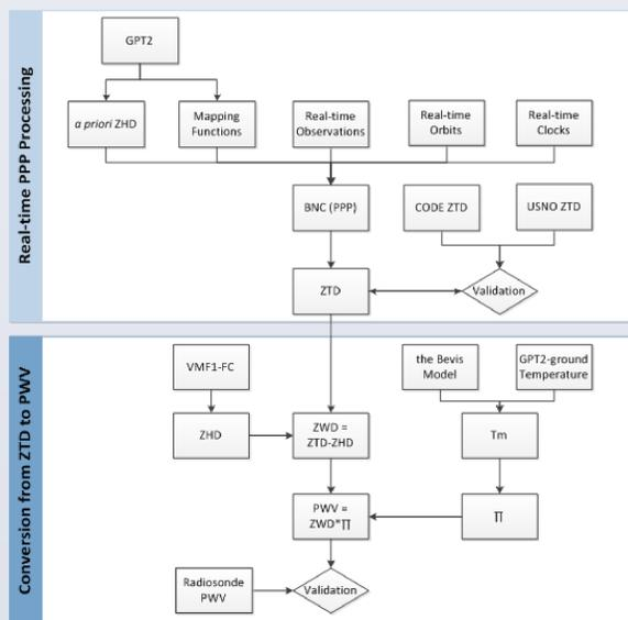
Fig. 1: Flow chart of real-time retrieval of ZTD and PWV using the PPP technique
