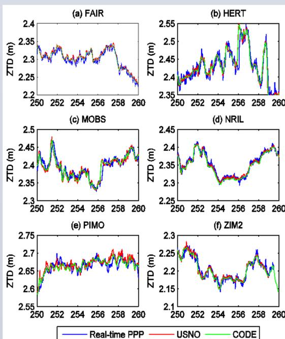
Fig. 3: ZTD from real-time PPP, USNO and CODE at six IGS stations during DOY 250-260, 2013. PIMO is a station where PPP-ZTDs show poorer agreement with the reference data. HERT is a station where real-time GPS data suffers from internet instability at the end of DOY 255. The other four stations are presented here for comparisons
